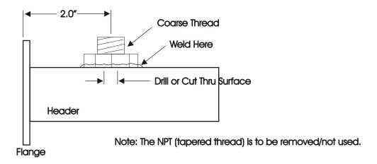
Alternately the entire larger thread diameter can be located inside of the exhaust header. The Hex Head will contact the outside surface of the exhaust header for welding
