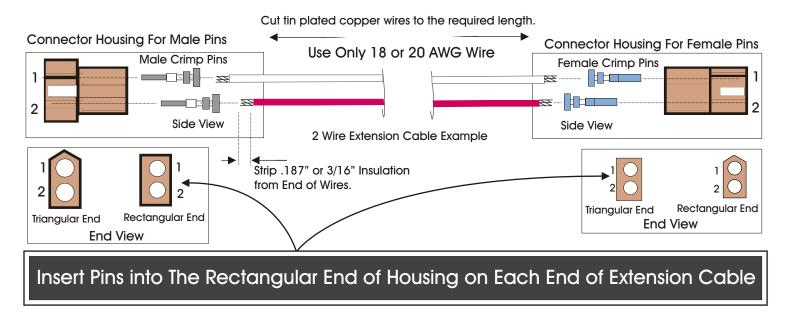
Push the Pin all the way into the housing, it will lock into position.
