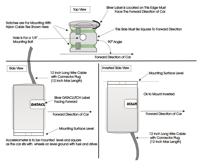
The NARROW SIDE or EDGE of the accelerometer WITH SILVER label MUST FACE IN THE CARS FORWARD DIRECTION..
