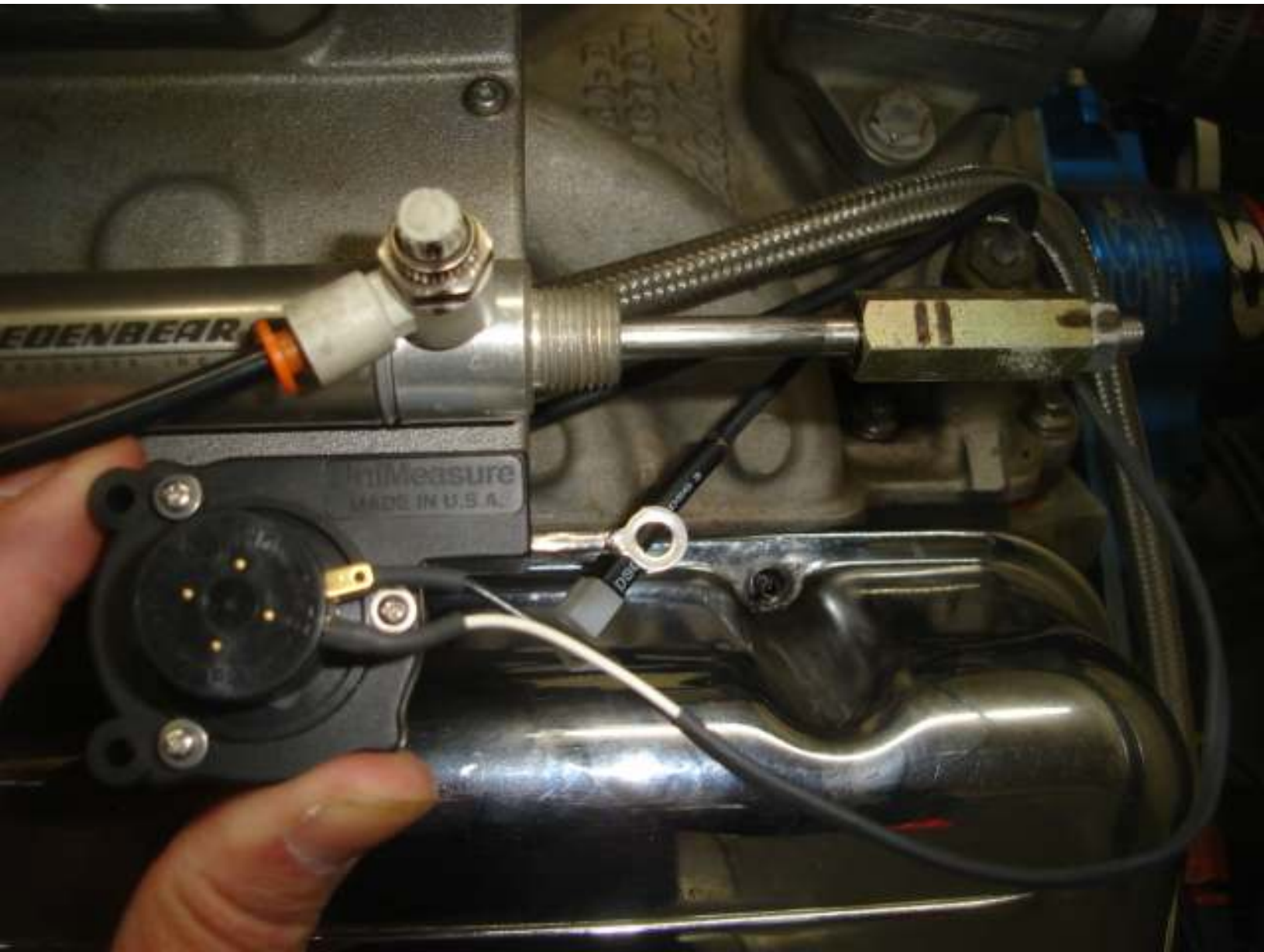
String Pot Position Sensor Located Near Throttle Stop
