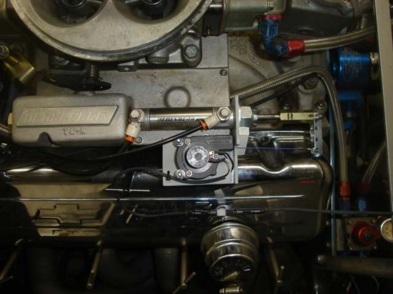
Position Sensor Held to Mounting Bracket with two 6-32 Machine Screws
